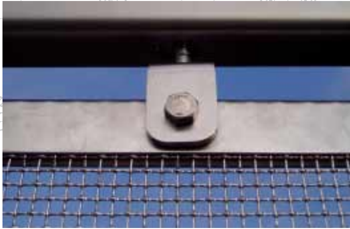
Top fixing: Tension profile and clevis screw
